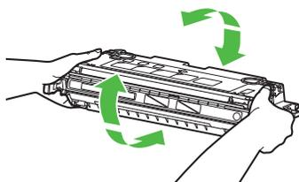
If toner is not distributed evenly, this may result in deterioration in print quality. Make sure to carry out this procedure properly.
