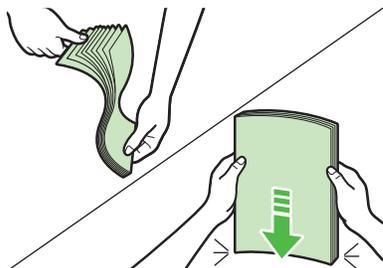
**10** Load the paper stack of the appropriate size with the print side facing up. Align the rear edge of the paper stack with the rear paper guide.
