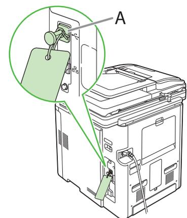
Remove the attachment (A) that covers the USB port on the back of the machine.
