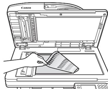
Place the test print face down on the platen glass, with the black bands along the top left edge of the platen glass. Stack approximately 20 sheets of blank paper on top of the test print for a more precise gradation correction.
