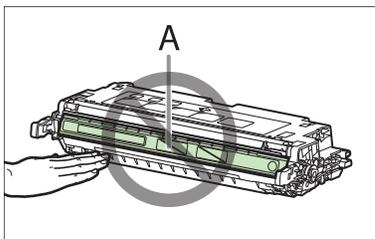
– Do not touch the high-voltage contact (A) or the electrical contacts (B), as this may result in damage to the printer.
