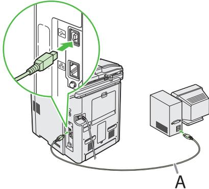
Connect the machine and your computer with a USB cable (A).
