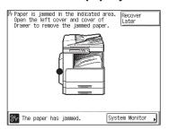
When you press [Recover Later], you can continue operations, such as setting modes and scanning originals, without removing the jammed paper immediately.
